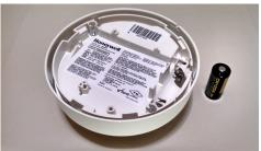
Remove old battery from sensor. The battery required for this model is part number **CR123**. Install new battery.
